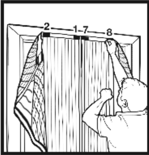
5. Repeat for hook and loop strips #2 and #8. Hold for 30 seconds. Note: Be sure to hang the screen high enough so that it does not drag on the ground.
