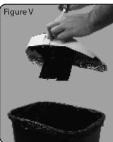
1. To empty the Hurricane® Spin Broom™ dust bin, hold it over a garbage can and push in the dust bin button to allow all of the contents to fall out. (Figure V) After everything has fallen out make sure to close the dust bin door.
