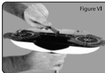
1. Periodically clean the center brush with the included brush cleaning tool. (Figure VI)
