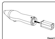
5. With the green arrows lined up, insert the battery cradle into the power handle. (Figure E)
