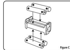
3. Insert 4 AA batteries according to the markings on the battery cradle. (Figure C)
