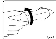
1. Turn the battery cap counter-clockwise to access the battery compartment. (Figure A)
