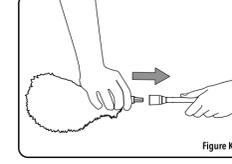
4. Now you can snap a dusting head onto the extension arm. (Figure K)
