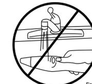
3. Never expose the Power handle to water. Wipe clean with a damp cloth. (Figure N)
