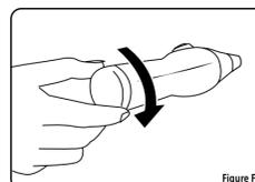
6. Turn the battery cap clockwise to lock the battery compartment. (Figure F)
