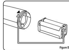
4. Line up the blue arrow on the power handle and the blue arrow on the battery cradle. (Figure D)
