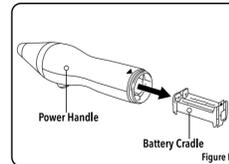
2. Pull the battery cradle out of the power handle. (Figure B)
