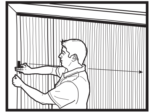
6. Attach the rest of the hook and loop strips row by row: #1-4 and #6-9 (Fig. 2)
