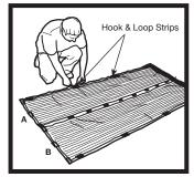
3. Peel the adhesive backing off of the hook and loop strips and apply to the Magic Mesh® Screen according to FIGURE 1.
