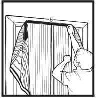
5. Place the remaining length of hook and loop strip #5.
