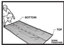
2. Lay your Magic Mesh® Screen flat on the floor with the magnets aligned in the center. **Note**: The top of the panel will have a larger gap between the magnets and the trim versus the bottom of the panel. The top strip of the panel is where side **A** and **B** are sewn together.
