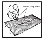
3. Peel the adhesive backing off of the hook and loop strips and apply to the Magic Mesh® Screen according to FIGURE 1. Note: Hook and Loop #5 is split into two separate strips
