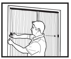
**6.** Attach the rest of the hook and loop strips row by row: #1-4 and #6-9. Figure 2
