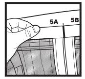
4. Peel off 1/2 adhesive backing of hook and loop strips then apply them to the door frame one at a time with pressure. Hold for 30 seconds. **Note:** Be sure to hang the screen high enough so that it does not drag on the ground.
