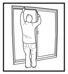
1. Find and mark the center point of the top of the opening door. Measure the opening of the doorway. **Note:** If the opening is less than 91.4 cms (36 inches), we suggest removing the sliding screen door.
