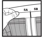
4. Peel off 1/2 adhesive backing of hook and loop strips then apply them to the door frame one at a time with pressure. Hold for 30 seconds.
